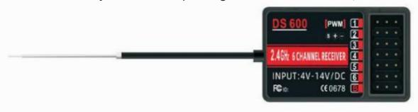
Note: The receiver's antenna is mainly used to receive signals. Please do not pull or cut the antenna during use. The receiver's antenna will receive stronger signals when it is in an upright state.
