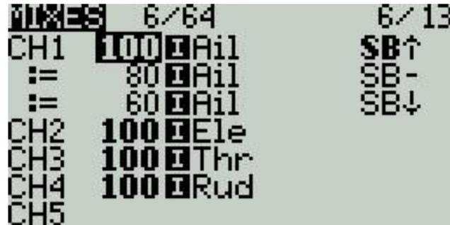
To edit a mixing control, use the scroll wheel to select the mixing control item up and down, and press and hold the ENT key to enter the editing submenu. Select Edit and press the ENT key momentarily.
