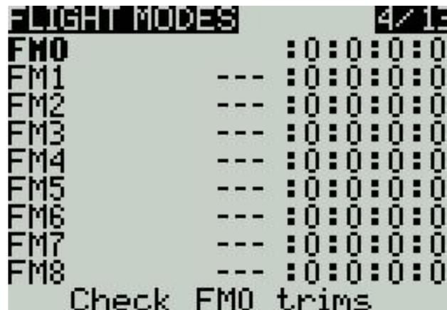
There are 8 flight modes plus the default FM0 available. The first item of FM1-FM8 requires a trigger switch. When no switch is on, FM0 is enabled by default.
