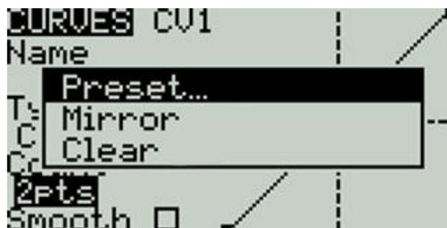
**Preset:** Select presets with slopes of  $-45^\circ$ ,  $-33^\circ$ ,  $-22^\circ$ ,  $-11^\circ$ ,  $0^\circ$ ,  $11^\circ$ ,  $22^\circ$ ,  $33^\circ$ ,  $45^\circ$ . When defining more complex curves, choose reasonable presets Will reduce some steps.
