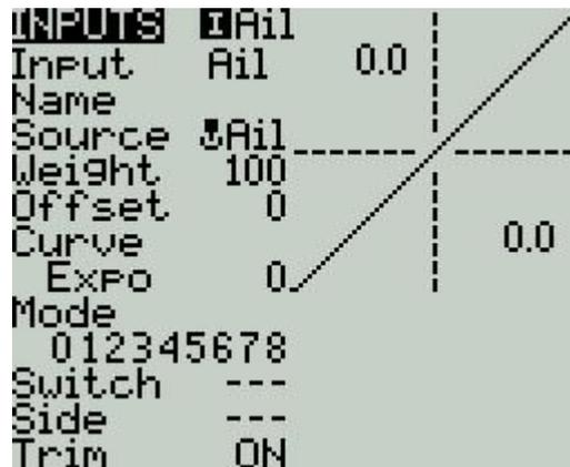
**Input name:** Name of the current entry. Use the scroll wheel to select a letter or number. Press and hold the ENT key to switch between upper and lower case. Press the ENT key to switch to the next character.
