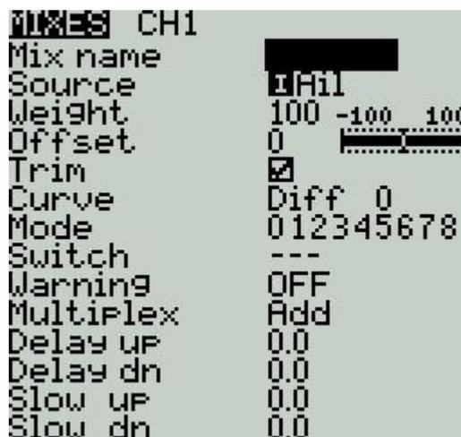
**Mix name:** Name setting Use the scroll wheel to select letters and numbers, and press and hold the ENT key to switch between upper and lower case. Short press the ENT key to set the next character.
