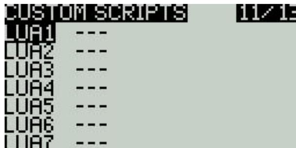
“ The Custom Scripts page is for mixed-type scripts that run continuously. These scripts should be placed in the / SCRIPTS / MIXE / folder of the SD card.
