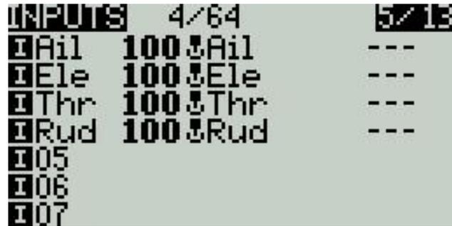
To set an entry, press and hold the ENT key on the current entry and a submenu will pop up
