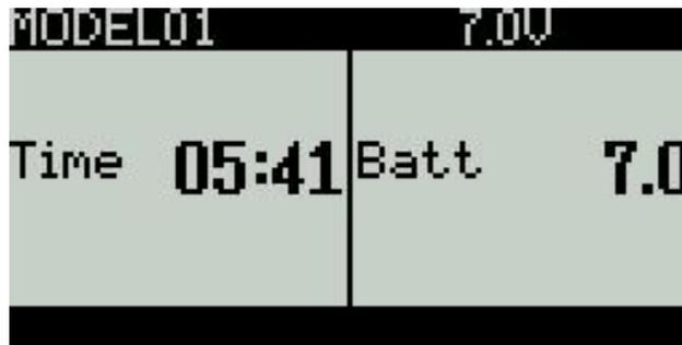
By pressing TELE from the main interface, vital telemetry information can be quickly displayed. Radiomaster has set two values- Time and Batt (system battery voltage) as defaults; these values can be changed by the user- displaying up to 4 values
