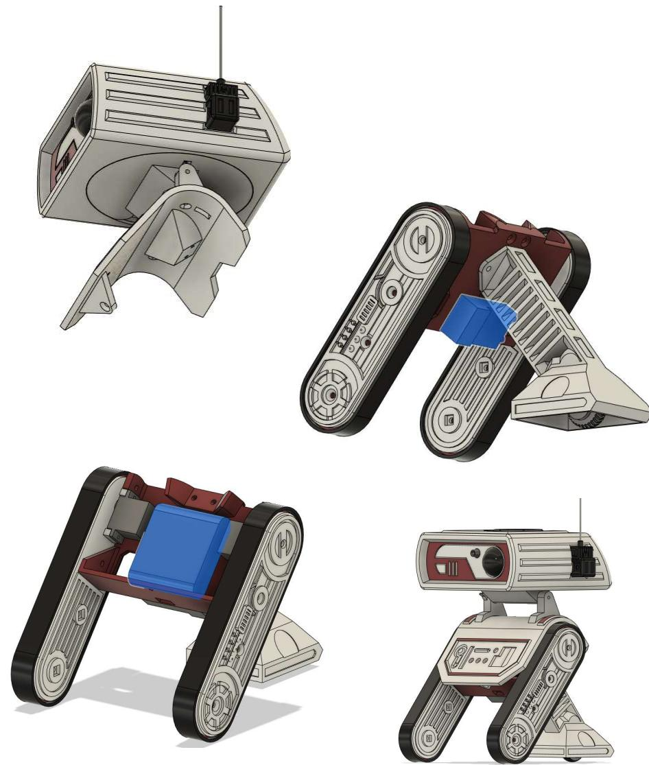
Take the head assembly and bolt this onto the BodyShoulder with M3x15 bolt (x2), note these self tap into the head brackets.
