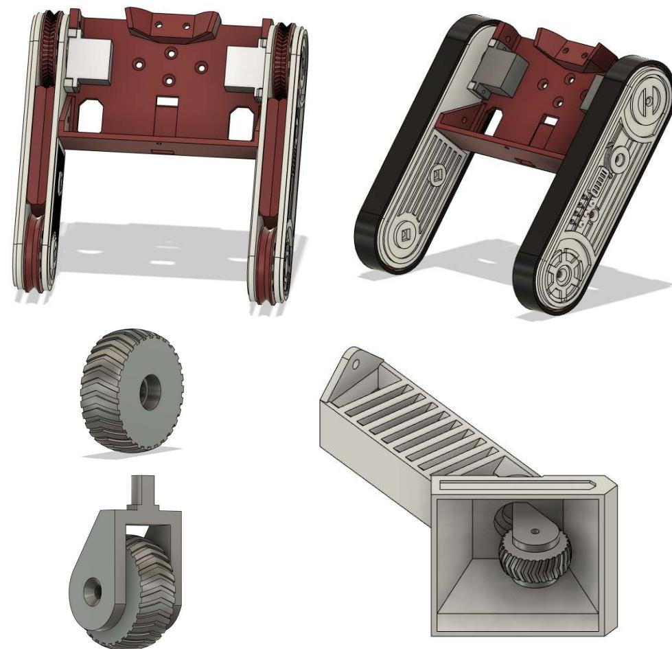
Once you've completed both sides, the assembly should look like this. Next take the two flex tyres and slip them over the two drive legs to finalise the drive system. The tracks are printed in soft TPU (I used Ninjaflex).
