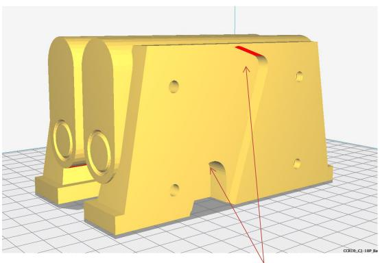
Battery Boxes printed vertical with supports needed in a few places, auto supports should be fine
