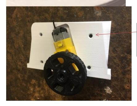
4 screws through from other side to screw into the side of each leg, no screw is required in the motor, a small step in the leg print holds the motor from sliding up.
