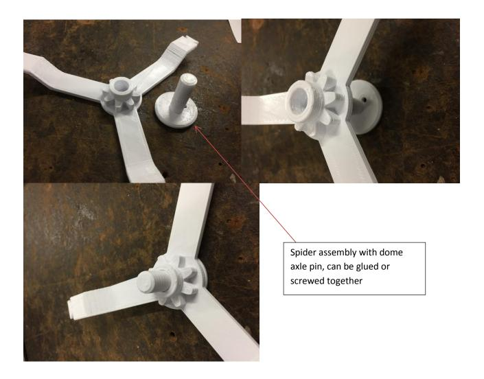
Carefully remove dome supports and file groove prior to painting
