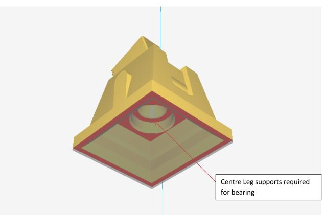
The dome and body are printed upside down with no supports, print at 0.2mm layer height for finer details.
