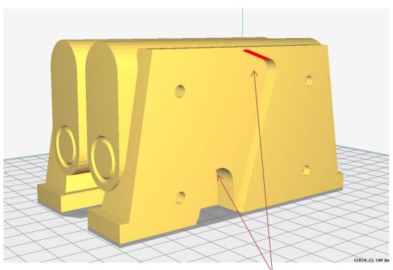
Battery Boxes printed vertical with supports needed in a few places, auto supports should be fine
