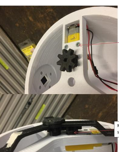
2 small screws retain motor, could be hot glued
