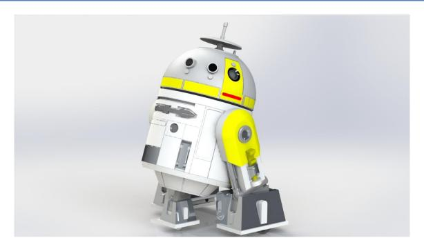
This is the guide for printing and assembling a mini CH-33P I designed, 3D printed body, simple electronics and controlled via Bluetooth smartphone app or your own device.
