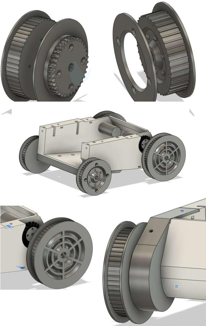
The front and rear wheels are assembled the same. The outer rim bolts onto the main wheel. On the larger wheel you use four M3x20 countersunk bolts, on the smaller wheel use four M3x10mm countersunk bolts. These just self tap into the plastic, tighten up firmly.
