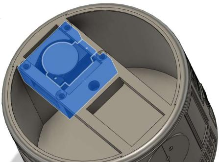
First, using the two screws which came with the servo, screw the FS90R servo into the FS90RFrame.
