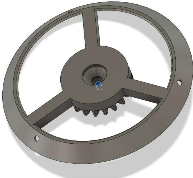
Take the dome ring and screw a M3x20mm countersunk bolt through the centre so it protrudes gear side.
