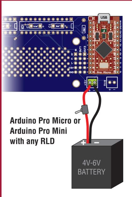
Arduino Pro Micro or Arduino Pro Mini with RLD V3.1
