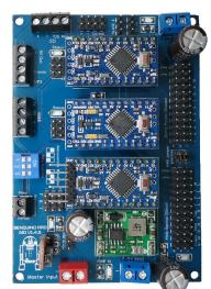
How is everything connected? Basically it's the "original" Marcduino Master/Slave & Flthy Wiring but all wires are replaced with traces and everything's on one pcb.
